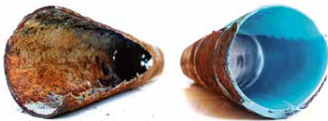
Pipe before and after Nu Drain treatment.
